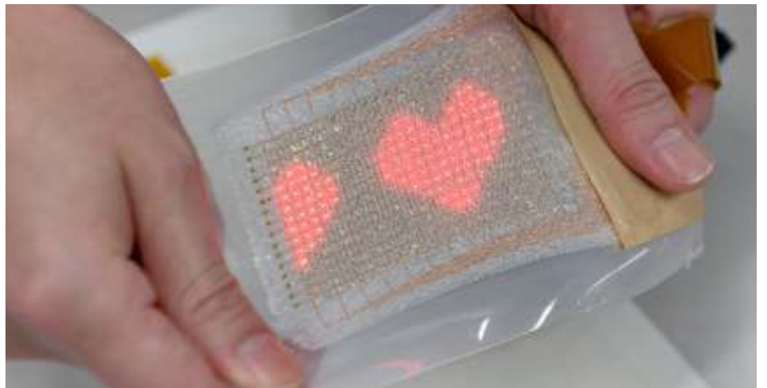
The band-aid-like device is just one millimetre thick and can monitor important health data as well as send and receive messages, including emojis.
